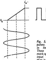
Fig. 5. Anode current pulses in "ideal" valve in limiting condition. These will have unity mark/space ratio if the input is much greater than is shown here.
