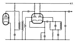
Above: Fig. 13. Practical circuit of synchrotector preceded by locked-oscillator limiter.
