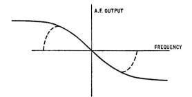
Fig. 7. A.F. output against frequency for gated-beam discriminator, assuming limiting at all frequencies. The dotted curve is that obtained in practice due to falling-off of signal amplitude with circuit selectivity.
