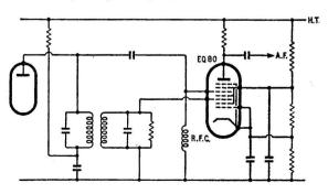
Fig. 3. Circuit for use with nonode discriminator.
